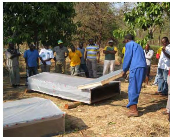
Showing how a solar drier works
