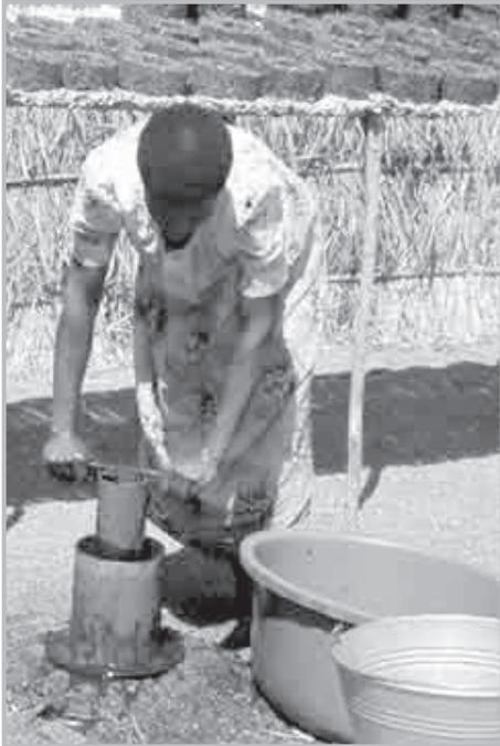
*Pressing briquettes. Notice the briquettes drying at the top.*
