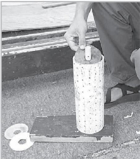
*PVC pipe with holes that allow the water to escape*
