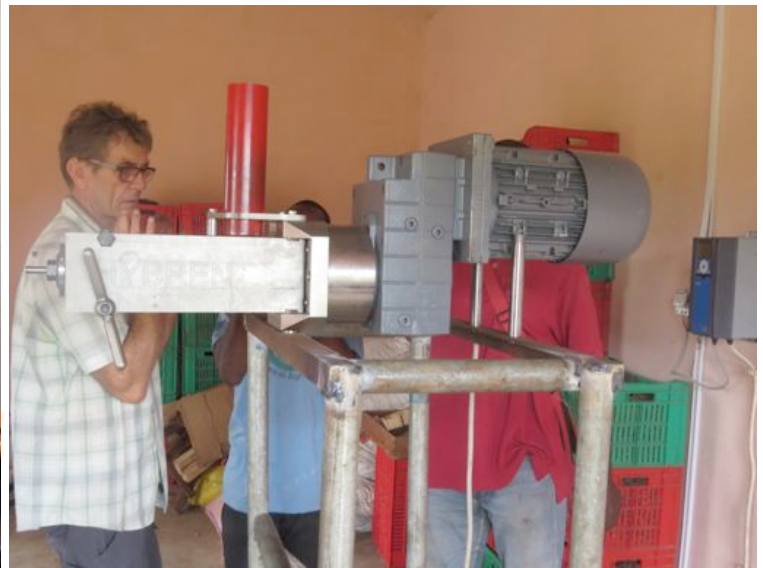
Installation and testing of the new jatropha oil presser bought from Denmark designed especially for pressing jatropha seeds.
